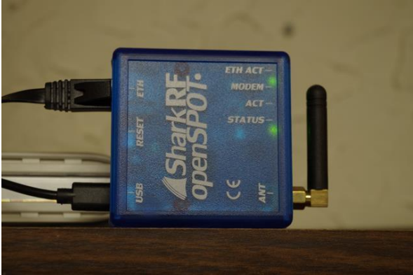
SharkRF OpenSpot (original). The original Openspot did not have WiFi. Later models added WiFi and removed the cabled ethernet capability.
