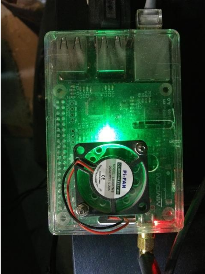
Raspberry Pi 3 with full size MMDVM board.
